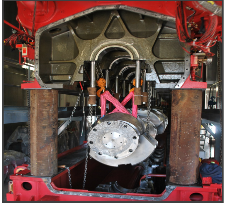
Crank Shaft Removal from Large Diesel Engine, Caribbean
